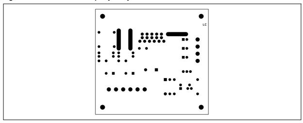
Figure 5. Evaluation Board Bottom Layer Layout
