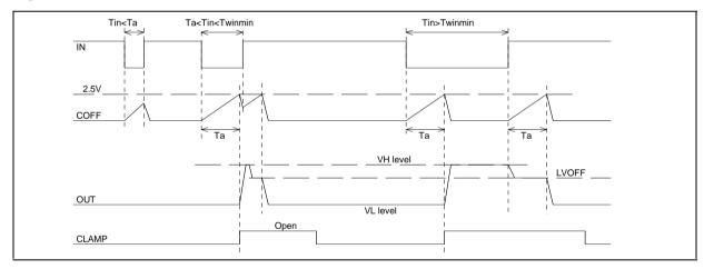
Figure 5: Desaturation fault
