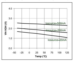
Figure 11: Desaturation source current vs temp.
