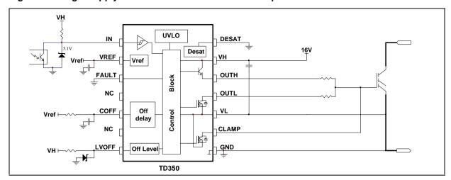
Figure 13: Large IGBT drive with negative gate drive and desaturation detection
