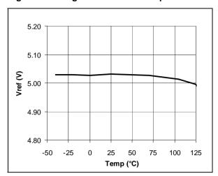
Figure 10: High level output voltage vs temp.
