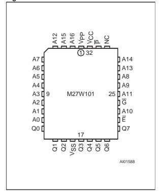
Figure 2C. TSOP Connections
