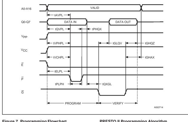
Figure 6. Programming and Verify Modes AC Waveforms
