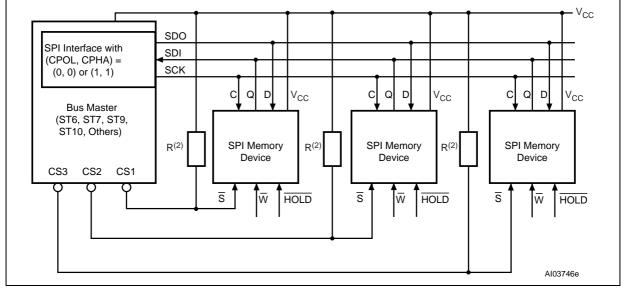
1. The Write Protect ( $\overline{W}$ ) and Hold ( $\overline{HOLD}$ ) signals should be driven, High or Low as appropriate.
