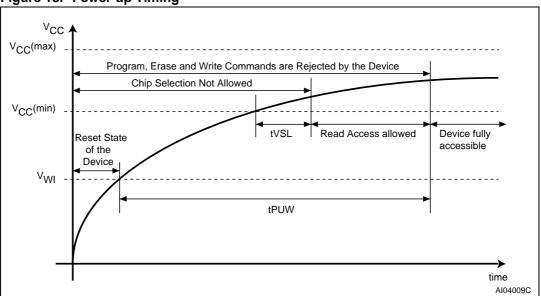
Figure 18. Power-up Timing
