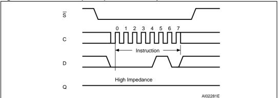
Figure 8. Write Enable (WREN) Instruction Sequence
