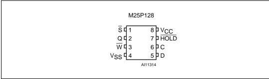
1. There is an exposed die paddle on the underside of the MLP8 package. This is pulled, internally, to  $V_{SS}$ , and must not be allowed to be connected to any other voltage or signal line on the PCB.
