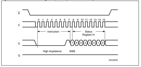
Figure 12. Write Status Register (WRSR) Instruction Sequence
