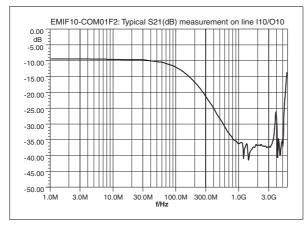
Note: Spikes at high frequencies are induced by the PCB layout
