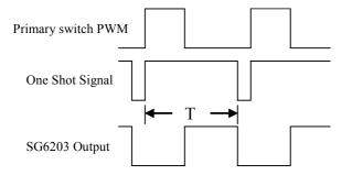
The on time of the synchronous MOSFET is then obtained by subtracting the on time of the primary switch from the one shot signal duration. If the resistor is too small, the synchronous MOSFET may be turned off even
