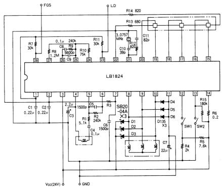
Unit (resistance:  $\Omega$ , capacitance: F)
