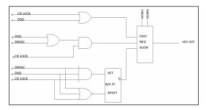
Figure 4. VDI Signal Response Configuration
