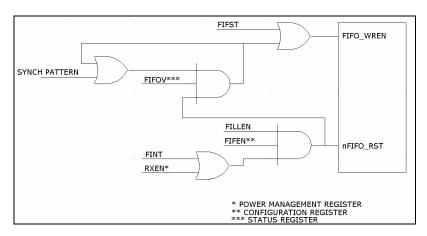
Figure 5. FIFO Write and Reset Configuration
