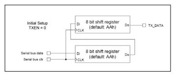
FIGURE 6. Initial TX Register Setting
