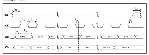
Figure 3. SPI Interface Timing
