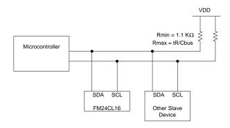
Figure 2. Typical System Configuration
