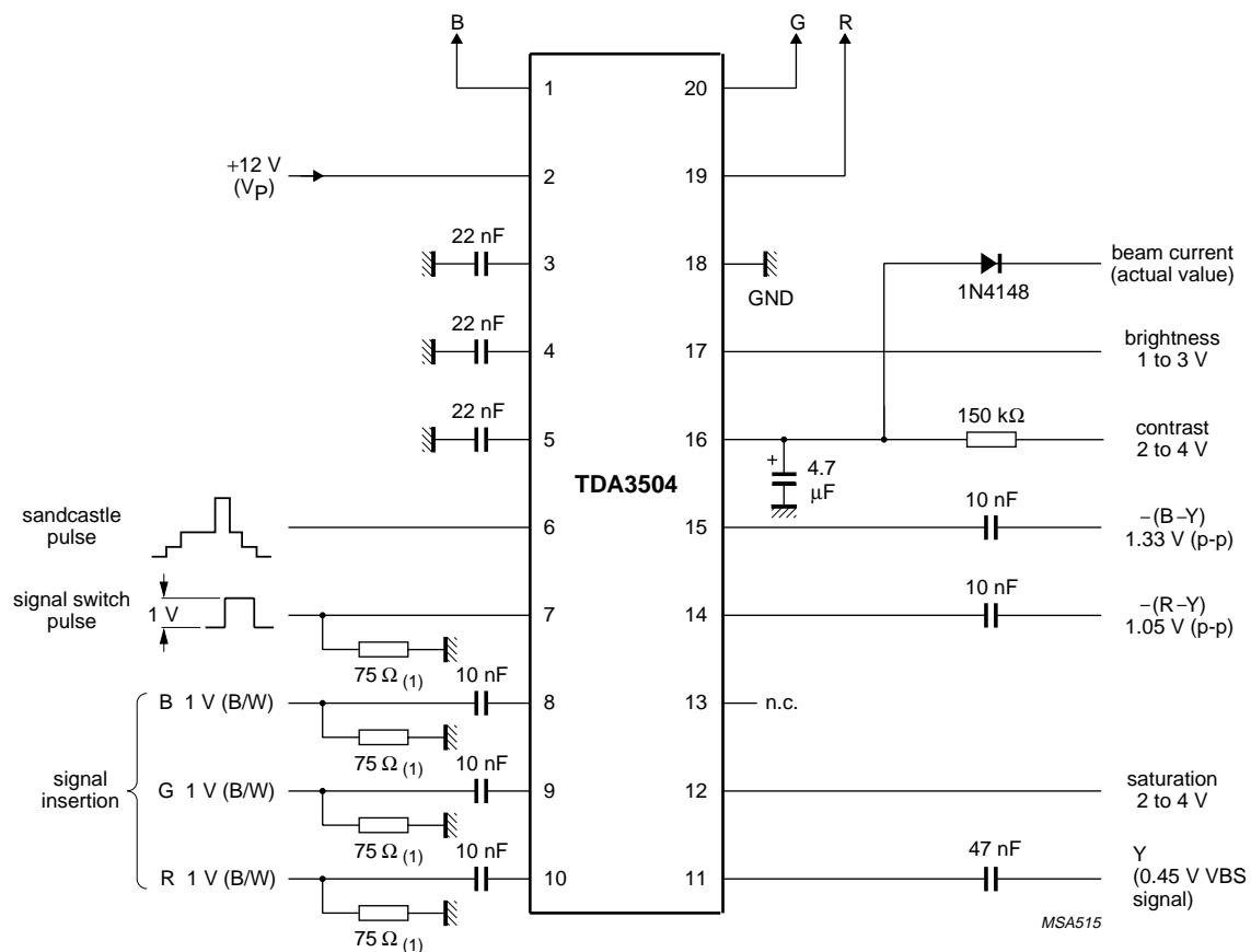
Fig.3 Basic application circuit diagram.
