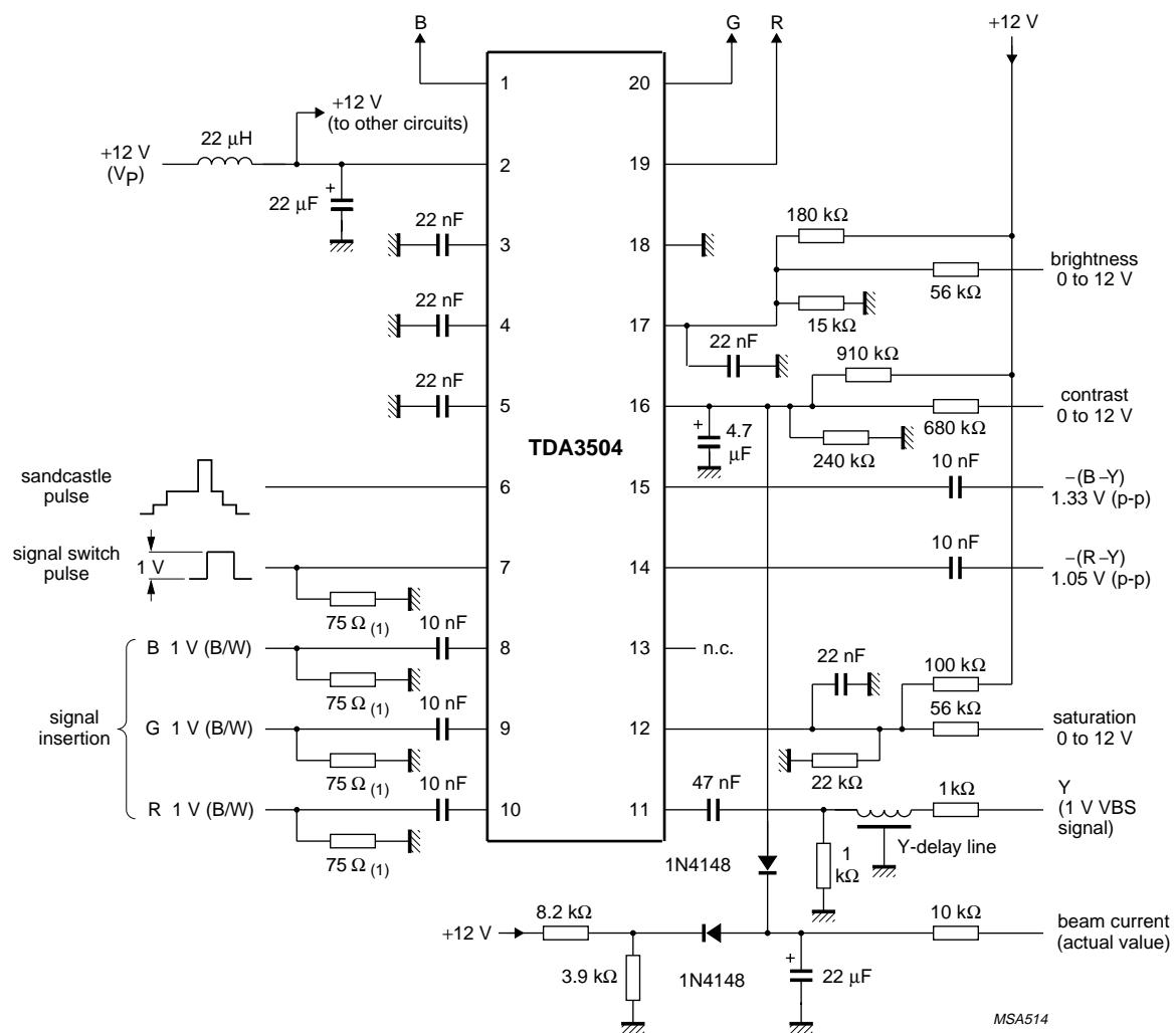
Fig.4 Typical application circuit diagram.
