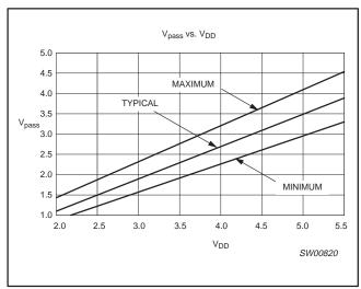
Figure 5. V<sub>pass</sub> voltage
