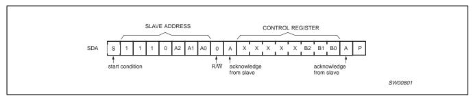
Figure 10. WRITE control register
