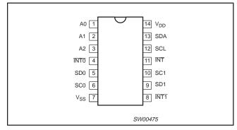
Figure 1. Pin configuration
