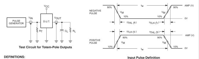
R<sub>L</sub> = Load resistor; see AC ELECTRICAL CHARACTERISTICS for value.
