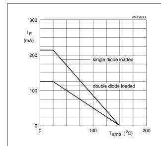
Device mounted on an FR4 printed-circuit board.
