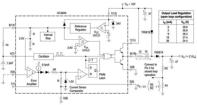
The capacitor's equivalent series resistance must limit the Drive Output current to 1.0 A. An additional series resistor may be required when using tantalum or other low ESR capacitors. The converter's output can provide excellent line and load regulation by connecting the R2/R1 resistor divider as shown.
