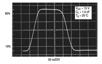
Figure 12. Output Waveform
