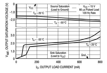
Figure 11. Output Saturation Voltage versus Load Current
