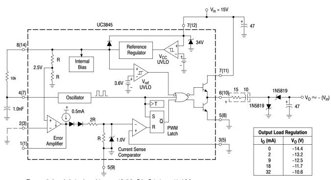
The capacitor's equivalent series resistance must limit the Drive Output current to 1.0 A. An additional series resistor may be required when using tantalum or other low ESR capacitors.
