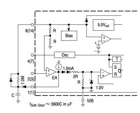
Figure 19. Adjustable Reduction of Clamp Level
