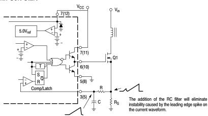
Figure 23. Current Waveform Spike Suppression
