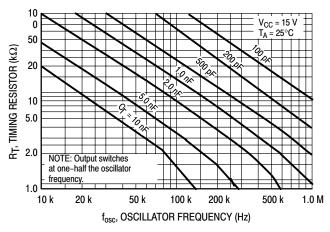
Figure 1. Timing Resistor versus Oscillator Frequency
