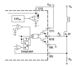
Series gate resistor  $R_{\rm g}$  will damp any high frequency parasitic oscillations caused by the MOSFET input capacitance and any series wiring inductance in the gate–source circuit.
