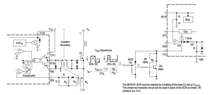
Figure 26. Isolated MOSFET Drive
