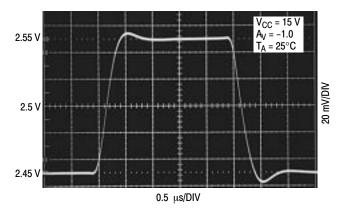
Figure 3. Error Amp Small Signal Transient Response
