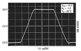
Figure 4. Error Amp Large Signal Transient Response
