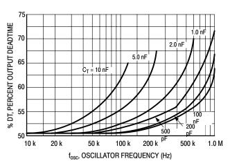
Figure 2. Output Deadtime versus Oscillator Frequency
