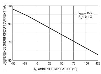
Figure 8. Reference Short Circuit Current versus Temperature
