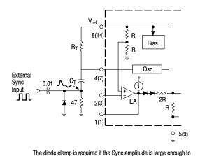
Figure 17. External Clock Synchronization
