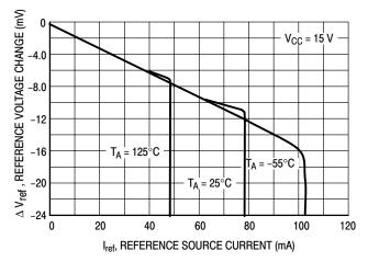
Figure 7. Reference Voltage Change versus Source Current
