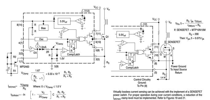
Figure 21. Adjustable Buffered Reduction of Clamp Level with Soft-Start
