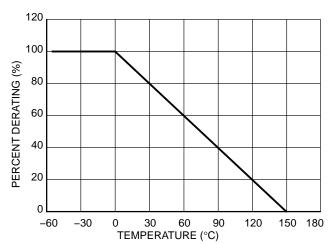
Figure 5. I<sub>R</sub> versus Temperature Characteristics of the NUP2105L
