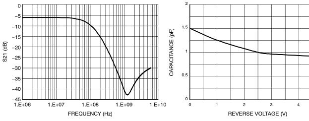
Figure 1. Insertion Loss Characteristic (Simulation)
