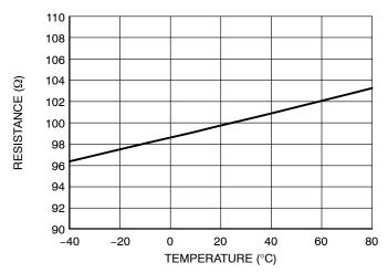
Figure 3. Typical Resistance over Temperature
