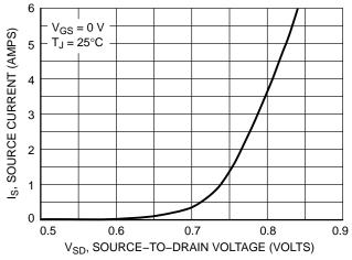
Figure 10. Diode Forward Voltage versus Current
