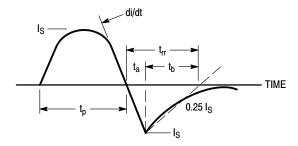
Figure 14. Diode Reverse Recovery Waveform
