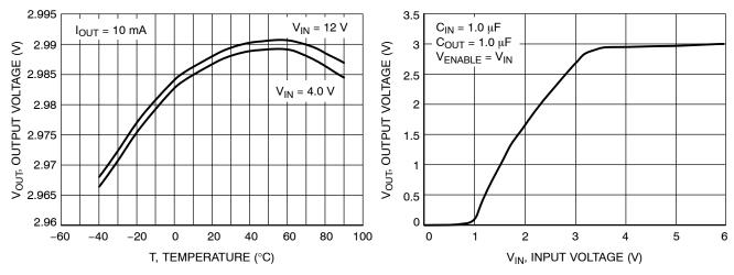
Figure 8. Output Voltage versus Temperature
