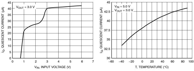
Figure 2. Quiescent Current versus Input Voltage
