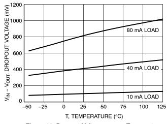
Figure 10. Dropout Voltage versus Temperature
