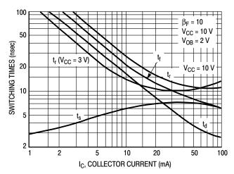
Figure 7. Typical Switching Times
