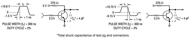
Figure 1. t<sub>on</sub> Circuit – 10 mA
