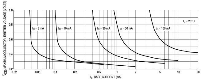
Figure 12. Maximum Collector Saturation Voltage Characteristics
