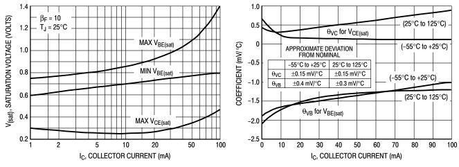
Figure 14. Saturation Voltage Limits
