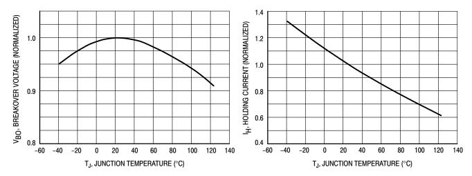
Figure 6. Typical Breakover Voltage
