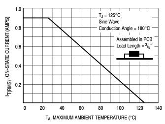
Figure 1. Maximum Lead Temperature
