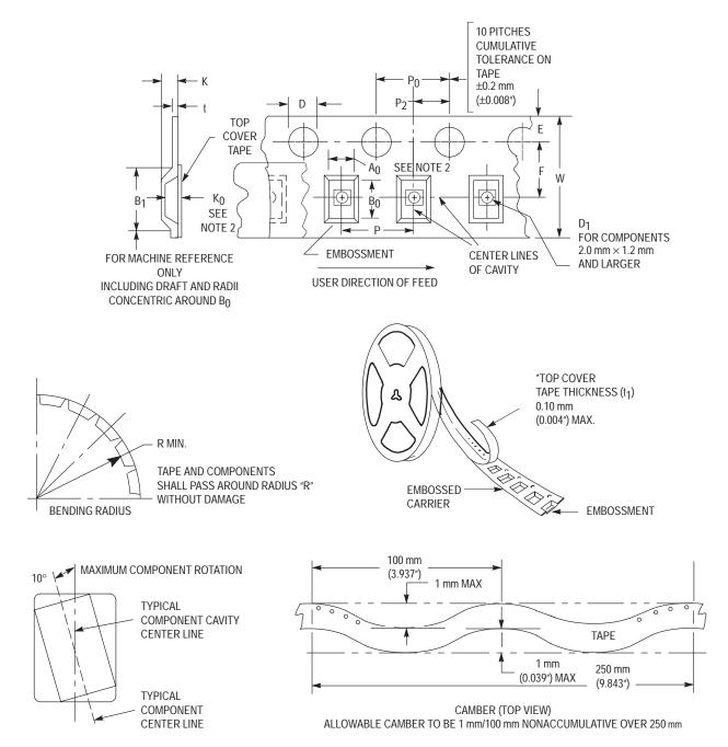
**Figure 4. Carrier Tape Specifications**
