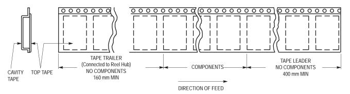
Figure 7. Tape Ends for Finished Goods
