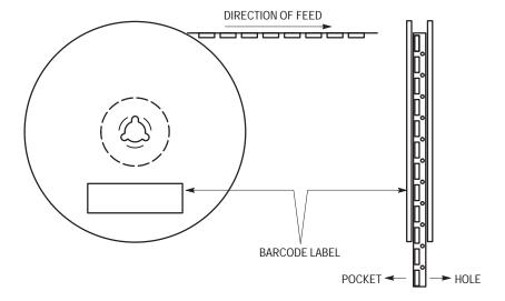
Figure 6. Reel Winding Direction
