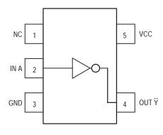
Figure 1. 5-Lead SOT-353 Pinout (Top View)
