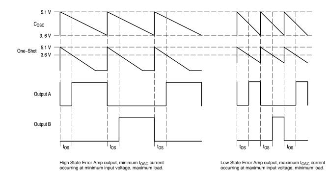
Figure 15. Timing Diagram
