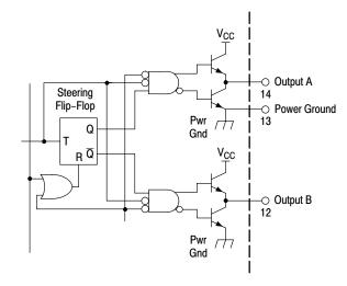
Figure 18. Steering Flip-Flop and Output Drivers
