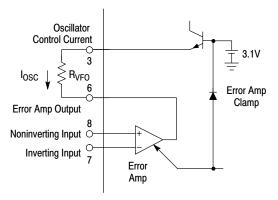
Figure 17. Error Amplifier and Clamp
