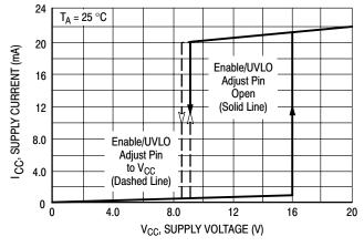
Figure 13. Supply Current versus Supply Voltage
