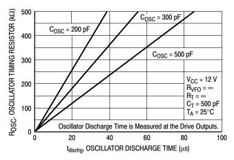
Figure 2. Oscillator Timing Resistor versus Discharge Time
