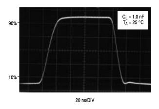
Figure 10. Drive Output Waveform
