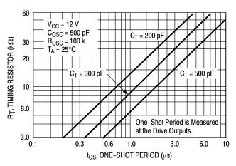
Figure 5. One-Shot Timing Resistor versus Period
