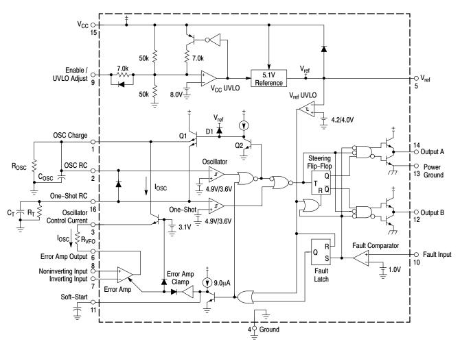
Figure 14. MC34067 Representative Block Diagram
