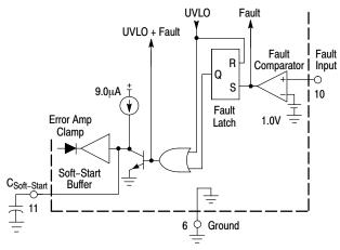
Figure 20. Fault Detector and Soft-Start
