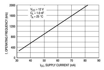
Figure 12. Operating Frequency versus Supply Current
