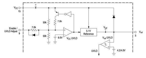
Figure 19. Undervoltage Lockout and Reference
