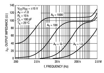
Figure 8. Output Impedance and Frequency
