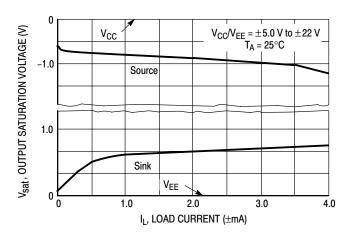
Figure 3. Split Supply Output Saturation versus Load Current
