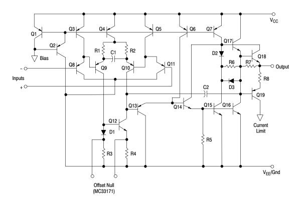
Figure 1. Representative Schematic Diagram (Each Amplifier)
