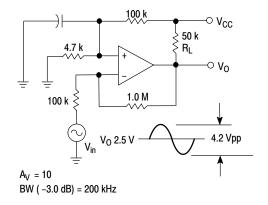
Figure 12. DC Coupled Inverting Amplifier
