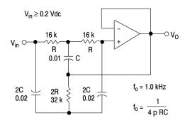
Figure 14. Active High-Q Notch Filter
