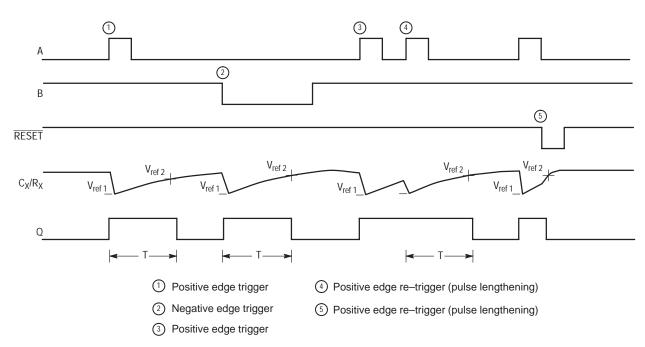
**Figure 10. Timing Operation**
