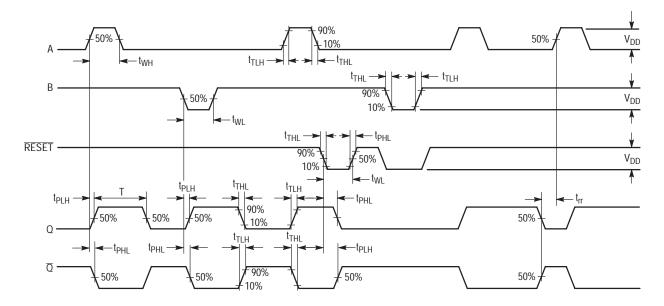
Figure 4. Switching Test Waveforms
