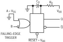
Figure 12. Retriggerable Monostables Circuitry
