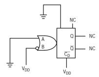
Figure 14. Connection of Unused Sections
