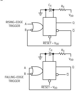
Figure 13. Non–Retriggerable Monostables Circuitry
