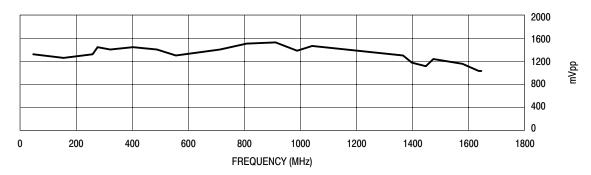
Figure 4. Output Amplitude versus Input Frequency
