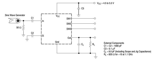
Figure 2. AC Test Circuit
