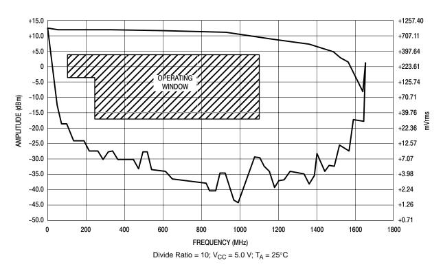
Figure 3. Input Signal Amplitude versus Input Frequency
