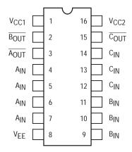
Pin assignment is for Dual–in–Line Package.
