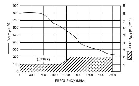
Figure 6. F<sub>max</sub>/Jitter
