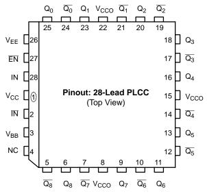
$<sup>^{\</sup>ast}$  All  $V_{CC}$  and  $V_{CCO}$  pins are tied together on the die.
