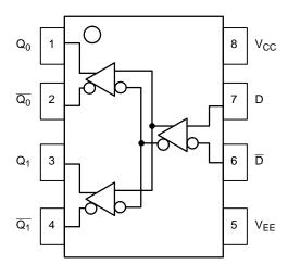
Figure 1. Logic Diagram and Pinout Assignment
