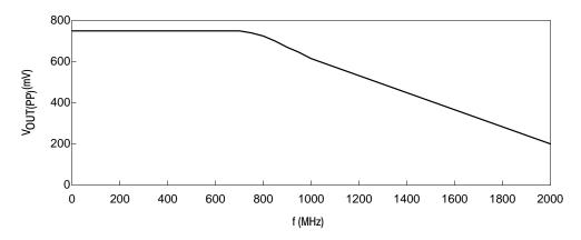
Figure 2. Output Swing versus Frequency
