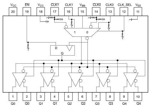
Warning: All  $V_{CC}$  and  $V_{EE}$  pins must be externally connected to Power Supply to guarantee proper operation.
