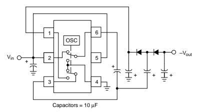
Figure 22. Negative Output Voltage Doubler
