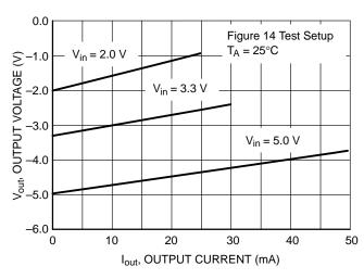
Figure 8. Output Voltage vs. Output Current
