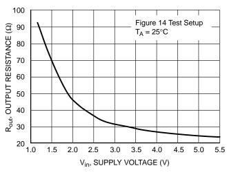
Figure 2. Output Resistance vs. Supply Voltage
