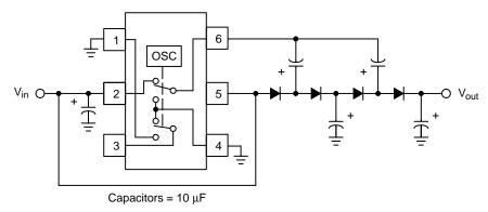
Figure 28. Positive Output Voltage Tripler
