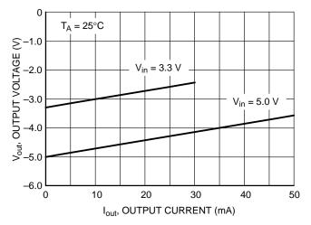
Figure 19. Inverter Load Regulation, Output Voltage vs. Output Current
