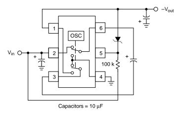
Figure 30. Load Regulated Negative Output Voltage
