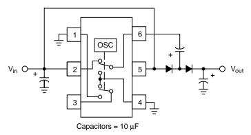
Figure 26. Positive Output Voltage Doubler
