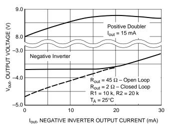
Figure 50. Load Regulation, Output Voltage vs.
