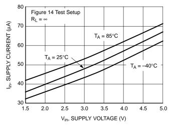
Figure 6. Supply Current vs. Supply Voltage
