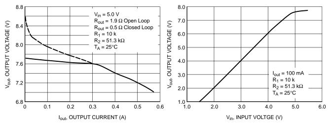
Figure 45. Current Boosted Close Loop Load Regulation, Output Voltage vs. Output Current
