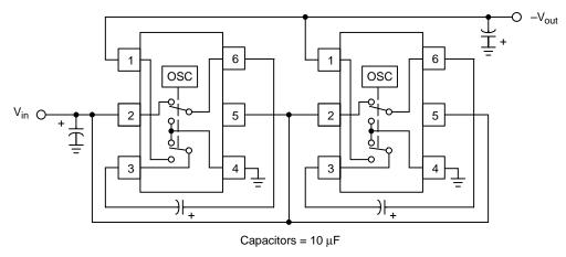
Figure 35. Paralleling Devices for Increased Negative Output Current
