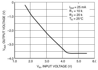
Figure 34. Line Regulation, Output Voltage vs. Input Current
