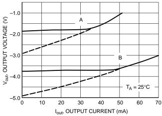
Figure 33. Load Regulation, Output Voltage vs.
