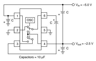
Figure 47. Negative Input Voltage Splitter
