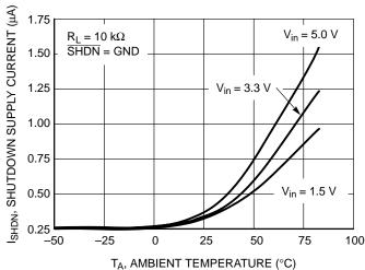
Figure 11. Shutdown Supply Current vs.
