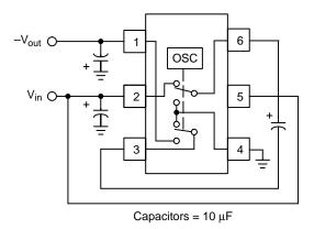
Figure 18. Voltage Inverter
