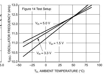
Figure 7. Oscillator Frequency vs. Ambient Temperature
