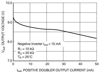
Figure 51. Load Regulation, Output Voltage vs.
