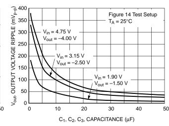
Figure 5. Output Voltage Ripple vs. Capacitance
