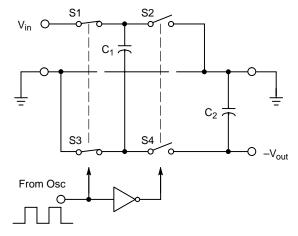
Figure 15. Ideal Switched Capacitor Charge Pump
