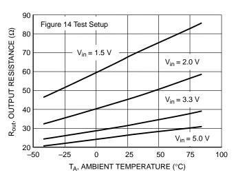
Figure 3. Output Resistance vs. Ambient Temperature
