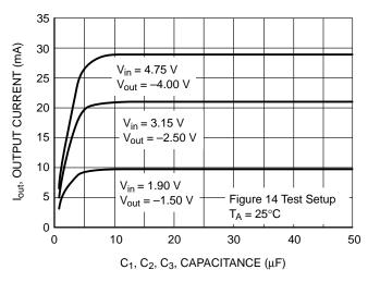
Figure 4. Output Current vs. Capacitance
