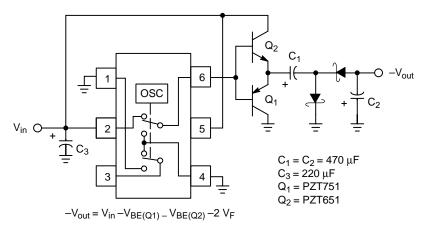
Figure 37. External Switch for Increased Negative Output Current
