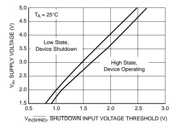
Figure 12. Supply Voltage vs. Shutdown Input Voltage Threshold
