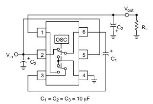
Figure 14. Test Setup/Voltage Inverter
