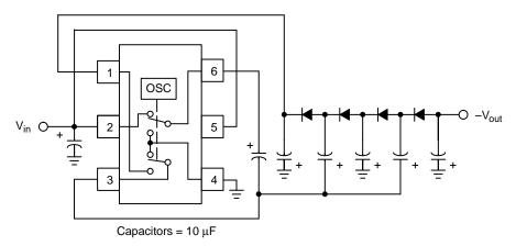
Figure 24. Negative Output Voltage Tripler
