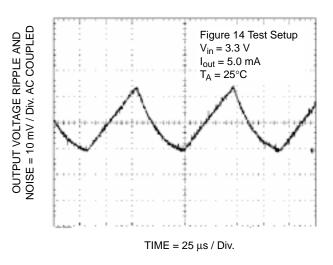
Figure 10. Output Voltage Ripple and Noise
