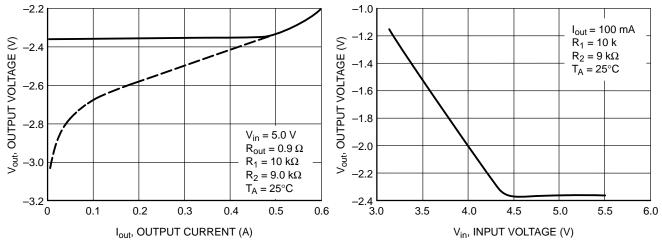
Figure 40. Current Boosted Load Regulation, Output Voltage vs. Output Current
