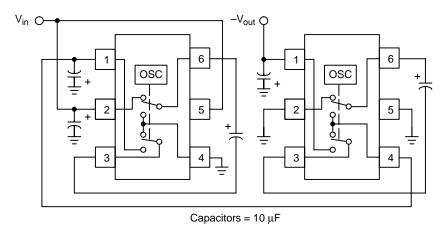
Figure 20. Cascaded Devices for Increased Negative Output Voltage
