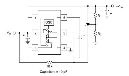
Figure 32. Line and Load Regulated Negative Output Voltage
