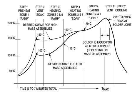
Figure 9. Typical Solder Heating Profile
