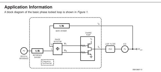
FIGURE 1. Conventional PLL Architecture
