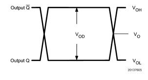
FIGURE 12. LVDS Output Signals
