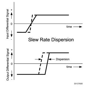
**FIGURE 7. Slew Rate Dispersion**
