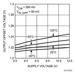
Differential Output Voltage vs. Supply Voltage
