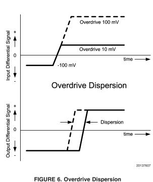
The overdrive dispersion is caused by the fact that switching currents in the input stage depend on the level of the differential input signal.
