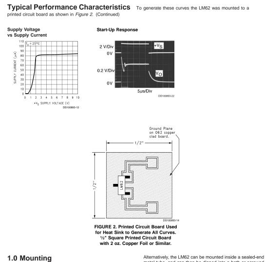
The LM62 can be applied easily in the same way as other integrated-circuit temperature sensors. It can be glued or cemented to a surface. The temperature that the LM62 is sensing will be within about +0.2°C of the surface temperature that LM62's leads are attached to.
