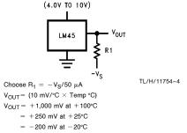
FIGURE 2. Full-Range Centigrade Temperature Sensor (-20°C to +100°C)
