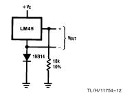
FIGURE 6. Temperature Sensor, Single Supply,  $-20^{\circ}\text{C}$  to  $+100^{\circ}\text{C}$
