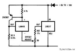
FIGURE 7. 4-to-20 mA Current Source (0°C to + 100°C)
