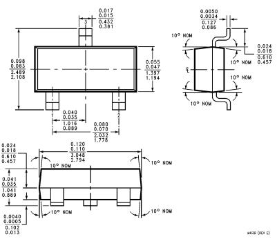
SOT-23 Molded Small Outline Transistor Package (M3)
