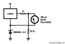
FIGURE 10. Expanded Scale Thermometer (50° to 80° Fahrenheit, for Example Shown)
