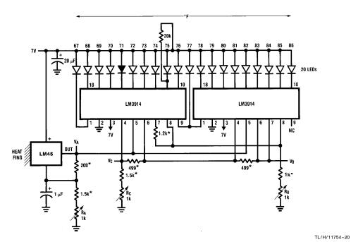
\*=1% or 2% film resistor -Trim R<sub>B</sub> for V<sub>B</sub>=3.075V -Trim R<sub>C</sub> for V<sub>C</sub>=1.955V -Trim R<sub>C</sub> for V<sub>A</sub>=0.075V + 100mV/°C  $\times$  Tambient -Example, V<sub>A</sub>=2.275V at 22°C
