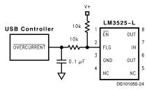
FIGURE 1. Transient Fitter
