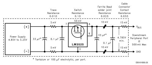
FIGURE 2. Self-Powered Hub Per-Port Voltage Drop
