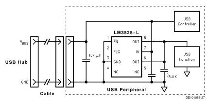
FIGURE 5. Inrush Current-limit Application
