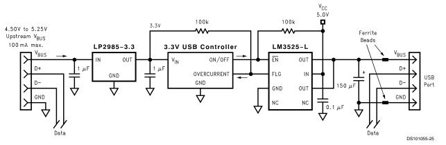
FIGURE 3. Single-Port USB Self-Powered Hub
