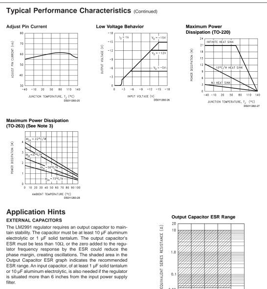
ESR range. An input capacitor, of at least 1 µF solid tantalum or 10  $\mu\text{F}$  aluminum electrolytic, is also needed if the regulator is situated more than 6 inches from the input power supply filter.
