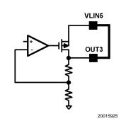
FIGURE 3. Connecting OUT3 to VLIN5 when not in use
