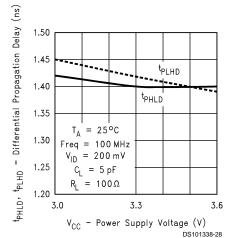
Differential Skew vs Power Supply Voltage
