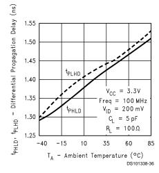
Differential Skew vs Ambient Temperature
