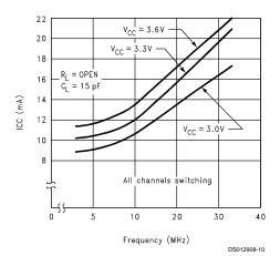
FIGURE 8. Typical  $I_{\text{CC}}$  vs Frequency
