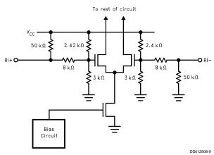
FIGURE 7. Typical Receiver Input Circuit
