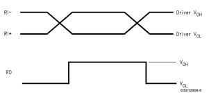
FIGURE 6. Typical Receiver Output Waveforms
