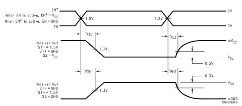
FIGURE 4. Receiver TRI-STATE Output Enable and Disable Waveforms (Notes 10, 11, 12, 13)
