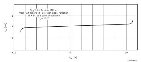
FIGURE 9. Receiver  $\mathbf{I}_{\mathrm{IN}}$  vs  $\mathbf{V}_{\mathrm{IN}}$  (Power On or Power Off)
