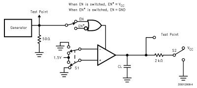
FIGURE 3. Receiver TRI-STATE Test Circuit
