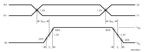
Note 10: Generator waveform for all tests unless otherwise specified: f = 1 MHz, Duty Cycle = 50%,  $Z_Q = 50\Omega$ ,  $t_r \le 10$  ns,  $t_l \le 10$  ns.
