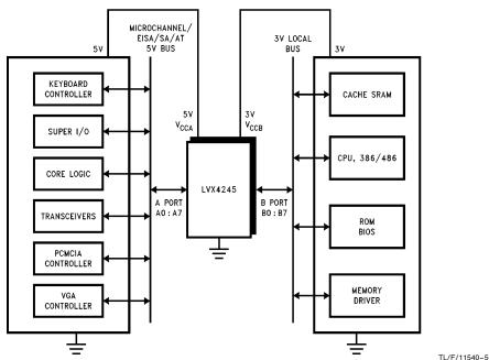
FIGURE 1. LVX4245 Fits into a System with 3V Subsystem and 5V Subsystem
