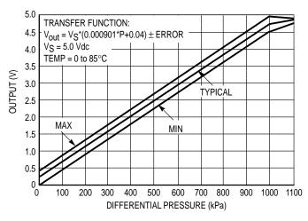
Figure 2. Output versus Pressure Differential
