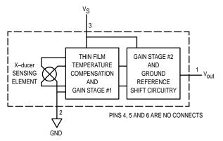
Figure 1. Fully Integrated Pressure Sensor Schematic
