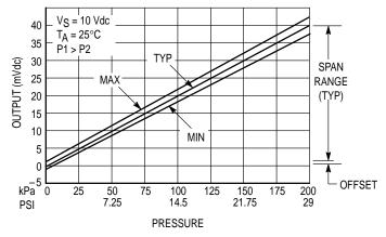
Figure 3. Output versus Pressure Differential
