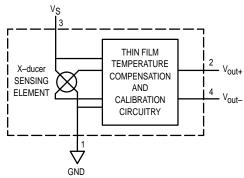
Figure 1. Temperature Compensated Pressure Sensor Schematic
