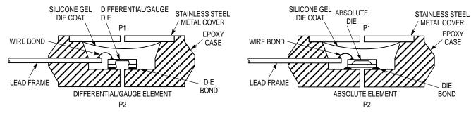
Figure 4. Cross-Sectional Diagrams (Not to Scale)
