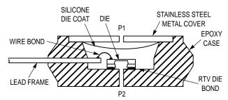
Figure 4. Cross-Sectional Diagram (not to scale)
