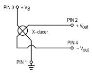
Figure 1. Uncompensated Pressure Sensor Schematic
