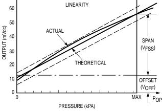
Figure 2. Output versus Pressure Differential
