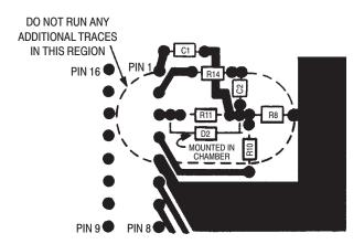
NOTES: Illustration is bottom view of layout using a DIP. Top view for SOIC layout is mirror image.
