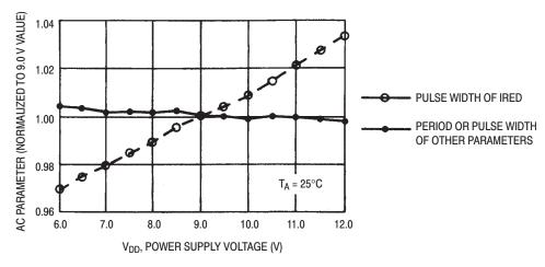
Figure 1. AC Characteristics versus Supply
