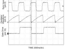
Figure 6. Sync Waveform
