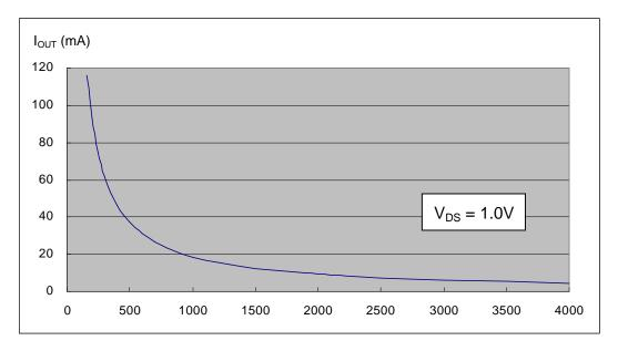
Resistance of the external resistor,  $R_{\text{ext}},$  in  $\Omega$
