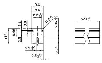
Tape and reel for SMT version - 1'000 relays / reel, 1'000 or 5'000 relays / box
