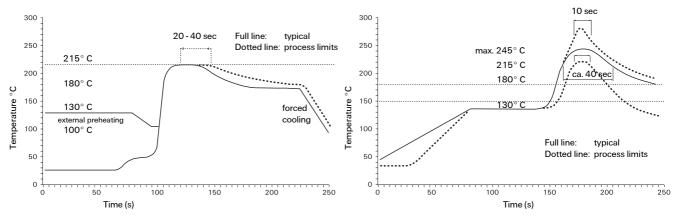
Vapor Phase Soldering: Temperature/Time Profile (Lead Temperature)
