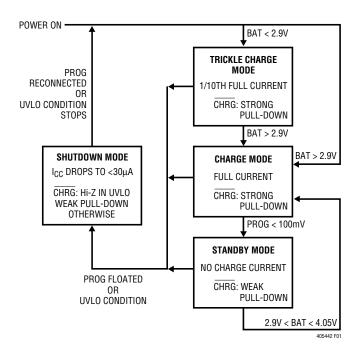
Figure 1. State Diagram of a Typical Charge Cycle
