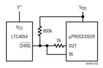
Figure 5. Using a Microprocessor to Determine CHRG State
