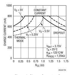
Figure 4. Charge Current vs R<sub>CC</sub>
