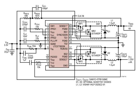
Figure 16. 2-Phase, Synchronizable, DDR Memory Supplies
