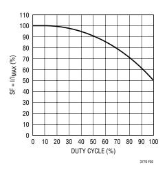
Figure 2. Maximum Peak Current vs Duty Cycle
