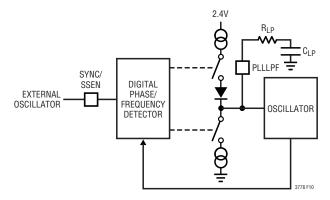
Figure 10. Phase-Locked Loop Block Diagram
