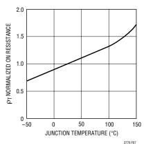
Figure 5. R<sub>DS(ON)</sub> vs Temperature
