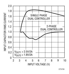
Figure 4. RMS Input Current Comparison
