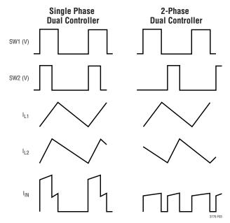
Figure 3. Example Waveforms for a Single Phase Dual Controller vs the 2-Phase LTC3776
