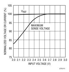
Figure 11. Line Regulation of V<sub>REF</sub> and Maximum Sense Voltage for Low Input Supply
