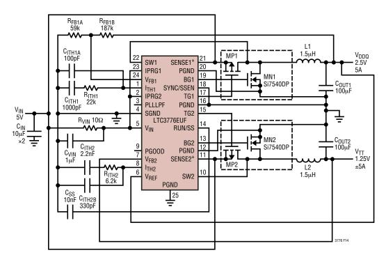
Figure 14. 2-Phase, 550kHz, DDR Memory Supplies
