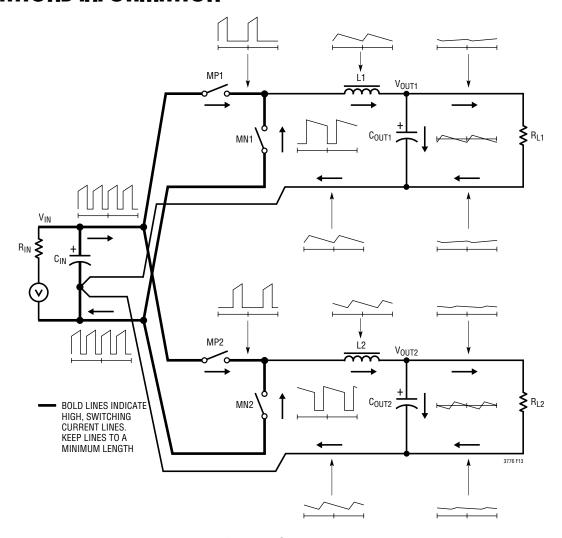
Figure 13. Branch Current Waveforms
