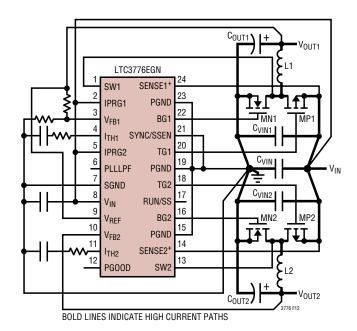
Figure 12. LTC3776 Layout Diagram
